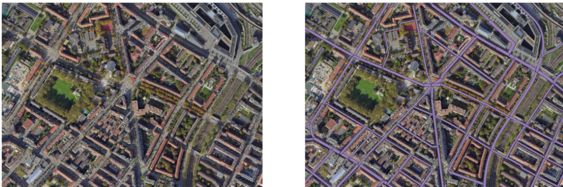
Figure 13.1: The aerial image (left) used as input to the machine learning model and the resulting road space estimation (right).
