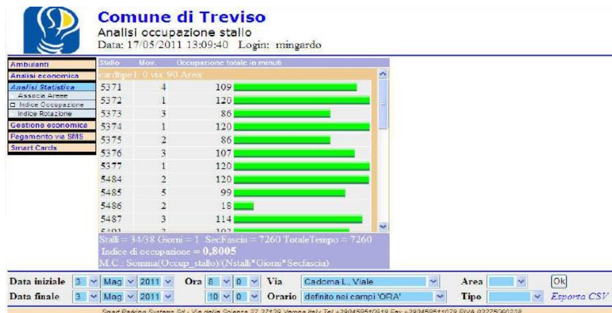
Figure 5: example of the data provided by the system: real time information about the occupancy ratio per parking lot.
