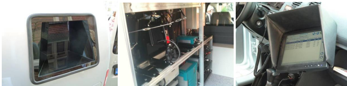
Figure 1: the scan-car; Left: the side of the scan car with cameras behind the mirrored glass. Middle: camera system inside the car. Right: the computer display showing information on the scanned license plates.
