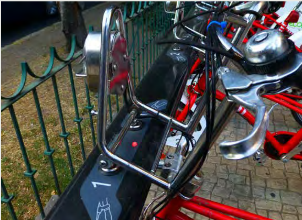
TOP In Rio de Janeiro's system, bikes lock into the side of the docking bar, rather than the top. AIMEE GAUTHIER
